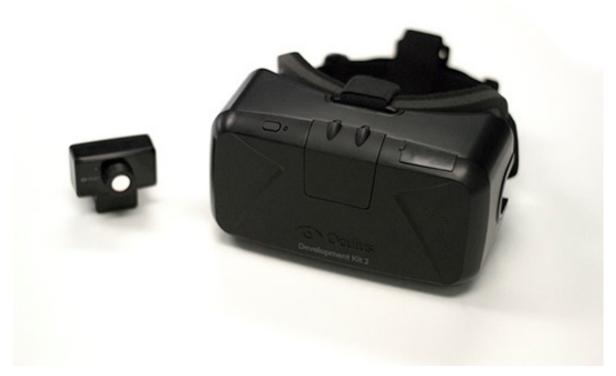
Figure 1. Oculus Rift version DK2 with movement capture camera. Source: [8].
