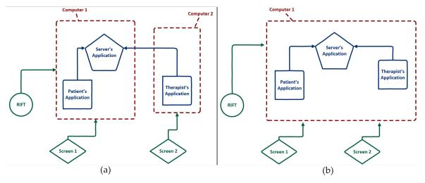
**Figure 2.** The images represent the two possible setups the system can accept, to be used in the OTs office. They differ in the number of computers (one or two). Configuration 1 (**a**) with two computers. Configuration 2 (**b**) with one computer and two screens.
